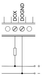
At some electrical loads connected to Digital output (such as external relay) it is appropriate to make use of flyback diode accessible through FBD screw connector. The following illustration depicts a connection of external relay to digital output while using integrated FBD diode.
