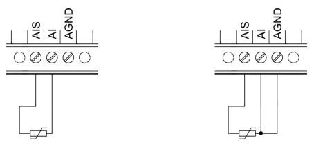
It is not possible to measure resistance sensors through Analog inputs in Group 1. Such measurement is possible to achieve trough connection to Group 1 analog outputs and also by using analog inputs of other groups.
