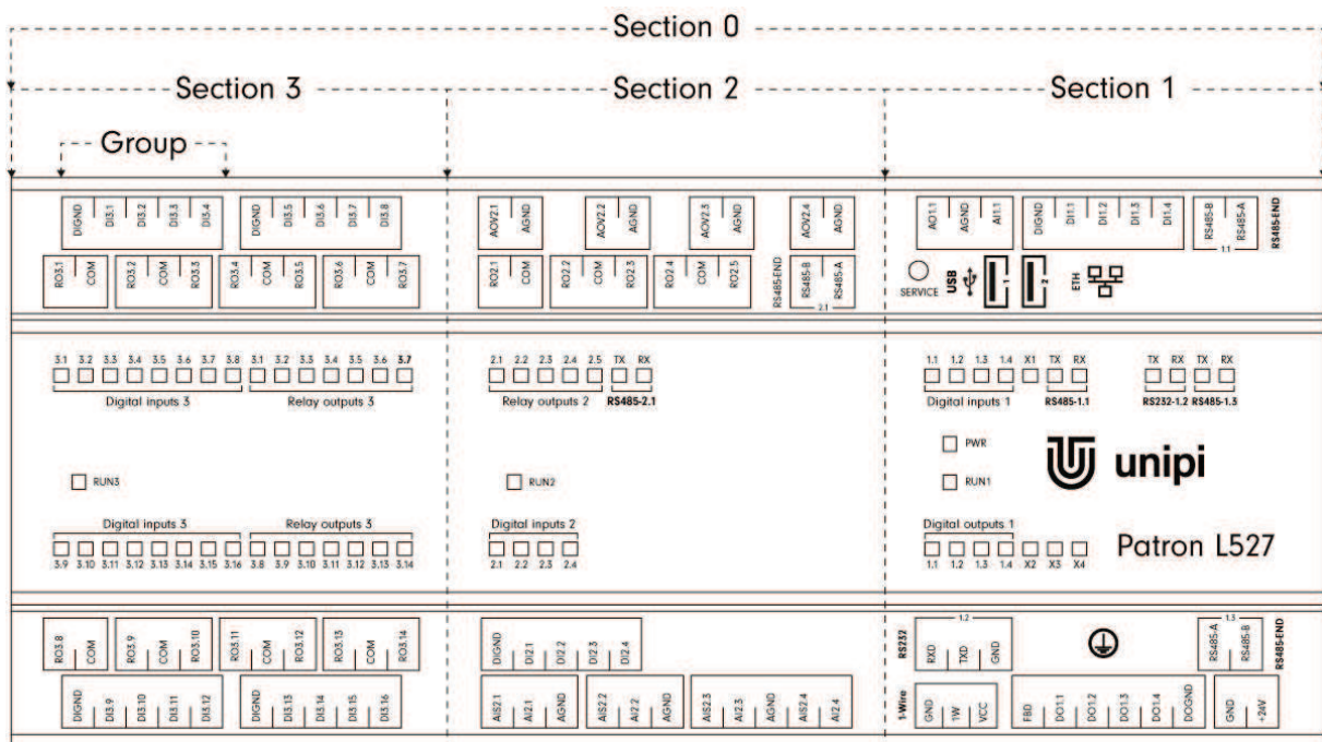
Example of numbering of inputs, outputs, groups and sections on the Patron L527 unit.
