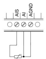
It is not possible to measure resistance sensors through Analog inputs in Group 1. Such measurement is possible to achieve trough connection to Group 1 analog outputs and also by using analog inputs of other groups.
