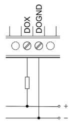
At some electrical loads connected to Digital output (such as external relay) it is appropriate to make use of flyback diode accessible through FBD screw connector. The following illustration depicts a connection of external relay to digital output while using integrated FBD diode.
